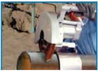
The Flex Track attaches to straight, contoured, cylindrical and serpentine surfaces for making accurate square cuts with no "HAZ".
