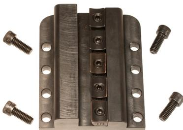
Tool Post and Tool Post screws
