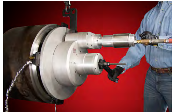
Compound bevel, face, and bore on 24" carbon steel pipe, 2" wall and wall variance of 1/4"
