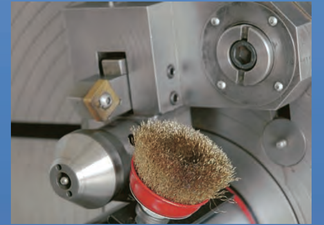
Tool slide, 30° bevel and ID cup brush
