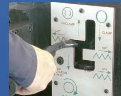
Single lever machine function control
