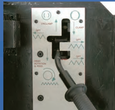
Pipeline machine control with rotation speed, feed, clamp pressure.
