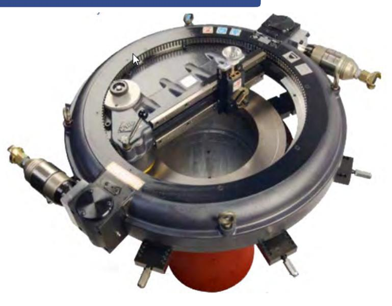
The SILK AX024 Rotary Machining Center is a larger version of the SX012 and has a maximum clamping capacity of 584mm (23"). It has an eight independent jaw clamping arrangement, and is driven by two 1.7kW (2.3hp) high torque pneumatic motors. The two continuous, automatic feeds offer a fine and a coarse surface finish
