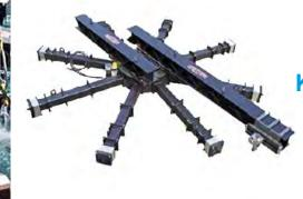
The MacTech LDFM 5000 Facing Machine is designed for on-site precision grinding, single point, mitering and rotary milling capabilities on large diameter flanges. Adjustable mounting legs secure the machine to the inside diameter of the workpiece.
