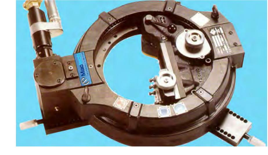
The Silk AXL0122 is a lightweight, portable, flange facing, grooving and weld preparation machine designed to machine full faced, raised face and grooved flanges from **0mm-305mm** (0"-12")
