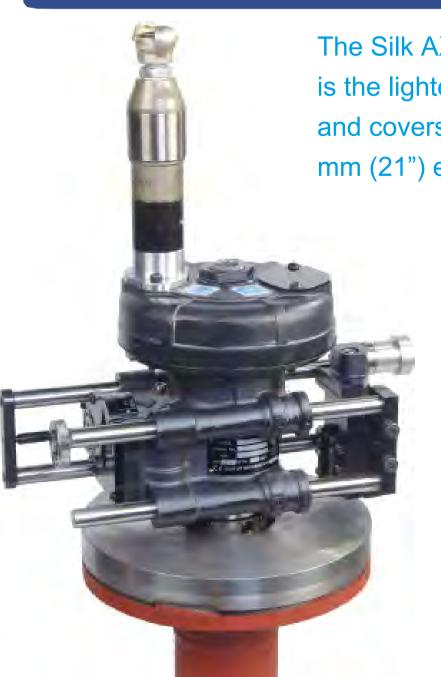
The Silk AX321 I/D Mounted Flange Facing Machine at 26.5kg (58lbs.) is the lightest flange facing machine in the Silk range. It is bore mounted and covers a range of flanges from 75 mm (3") internal diameter to 533 mm (21") external diameter.
