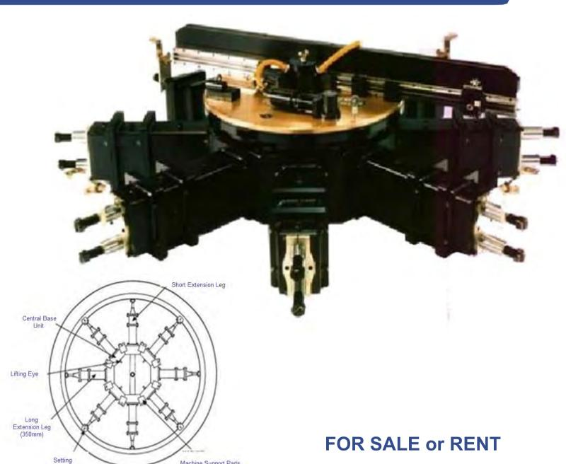
This SILK AX48120 is currently the largest internally mounted machine in our range. It can mount inside flanges having 1219mm (48") bores and can machine out to over 3048mm (120") in diameter.
