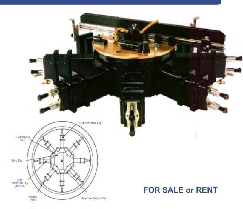
This SILK AX48120 is currently the largest internally mounted machine in our range. It can mount inside flanges having 1219mm (48") bores and can machine out to over 3048mm (120") in diameter.
