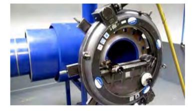
• Cuts "O" Ring grooves, RTJ and other V grooves, standard and compact flange facings,
