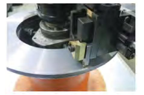
• Cuts "O" Ring grooves, RTJ and other V grooves, standard and compact flange facings, weld preparations, etc.
