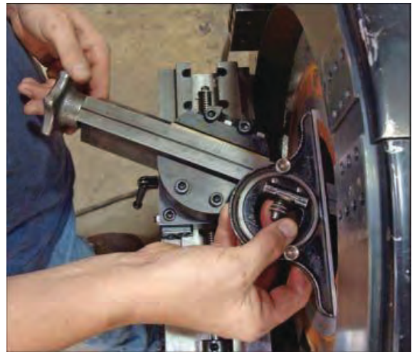
Adjustable Angle Tool Holder
