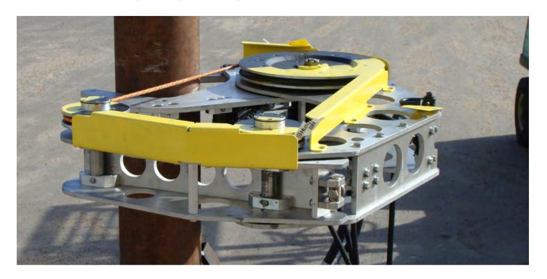
16 inch Cut-Off Diamond Wire Saw Stainless Steel Fittings & Fasteners
