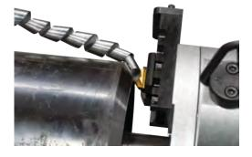
NOTE: Adjustable tool posts cannot be used in conjunction with conventional Blade Blocks that come standard with Commander, Dictator and Dictator II MILLHOGs. Simultaneous preps (bevel, face, bore) will require multiple adjustable tool posts
