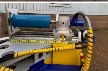
The existing method for topside/subsea core drilling and diamond wire cutting utilises a machine for each operation, diamond wire saw for cutting and dual drilling machine for drilling.
