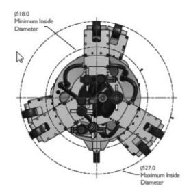
Machine is shown in the operating position.set for 27 inch diameter
