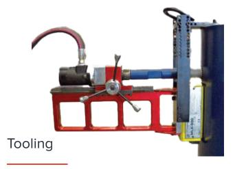
Mactech carries a full line of drill bits for most drilling operations. Drill capacity is 1-1/2 inch twist and 3 inch annular.
