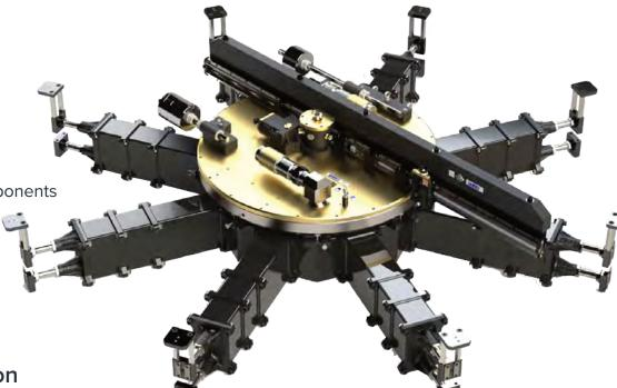
The AX48-120 Flange Facing Machine is designed to machine full face, raised face and grooved flanges from 1220mm to 3048mm (48" to 120") in diameter at any location having a minimum pneumatic air supply of  $5.8 \, \text{m}^3\text{/m}$  at  $6 \, \text{bar}$  (205 cfm, 90 psi)
